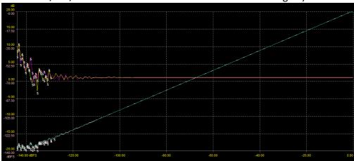
The Green line shows the absolute linearity. The Pink/Yellow line shows the abberation from linearity (digital signal generated by analyser and measured back by analogue inputs of analyser), where smaller deviations are better.
