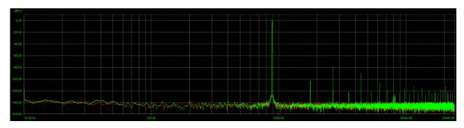
Input digital signal is OdBFS at 882 Hz (Red = right, Green = left). The lower the noisefloor, the better. The residuals inherent to NOS conversion are on the right side and measure -100dB for the  $2^{nd}$  harmonic and -80dB for the  $3^{rd}$  harmonic.
