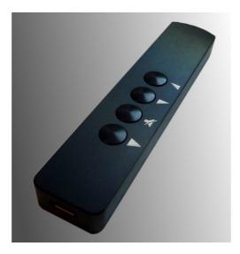
The remote control is made to control the available digital inputs, volume and muting. As opposed to the front panel buttons were you can select one of the digital sources directly , the remote will toggle through the entire range of available digital sources.
