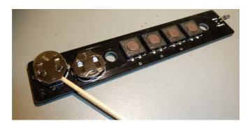
By turning the housing upside down the printed circuit board will fall out and the component side will be visible now. Remark: In case that the pcb is stocked in the housing you can push one of the buttons to help this procedure.
