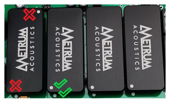
Again, the DAC3 modules need to be oriented with the dot on the module matching the dot on the circuit board.
