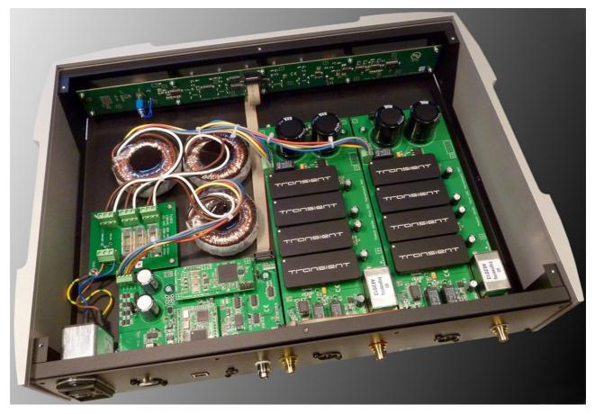
The digital input board (lower left) shows the difference; it has the forward correction module on it. Also, the DAC modules are DACone (check underside of module).
