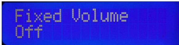
Rotate the Volume knob clockwise until the display shows the “On” status. Next press the volume knob to enter this new setting into the memory.
