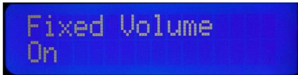
The new setting will be visible and where the “F” stands for “Fixed” Leave the menu by pressing the front panel source button.
