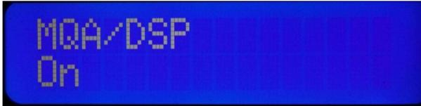
Turn the volume knob counter clockwise to switch the “MQA/DSP” function to Off. Rotating the volume knob clockwise will activate the “MQA/DSP” setting again. Press the volume knob to enter this setting in the memory of the Pasithea.
