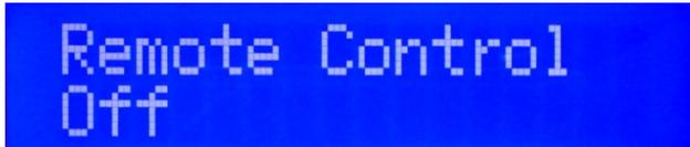
Enter the menu option. Turn the volume knob counter clockwise to switch the "Remote Control" function to Off. Rotating the volume knob clockwise will activate the "Remote Control" setting again. Press the volume knob to enter the desired setting in the memory of the Pasithea.
