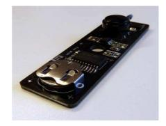
By turning the housing upside down the printed circuit board will fall out and the component side will be visible now.
