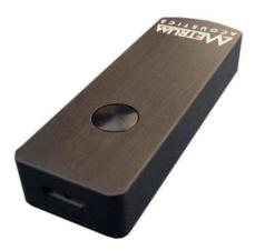
The remote control is made to control the available digital inputs. As opposed to the front panel buttons were you can select one of the digital sources directly, the remote will toggle through the entire range of available digital sources.
